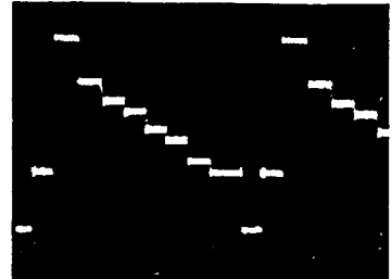
③ COLOR BURST SIGNAL (50mV/10ms) Pin ③⑤ of IC301 (0.5Vp-p)
